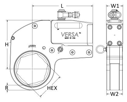
LEGEND: H = HEIGHT **W1** = WIDTH OF POWERHEAD **W2** = WIDTH OF LINK L = LENGTH R = DISTANCE FROM HEX CORNER
